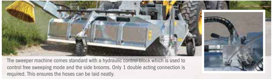
Powerful internal drive motor drives the sweeper roller directly and ensures neater sweeping close to the kerbside.
