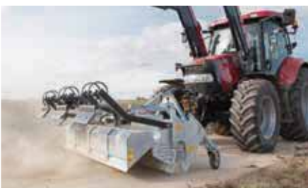
KEH type 500 on the front hydraulics with free sweeping mode and scraping device
