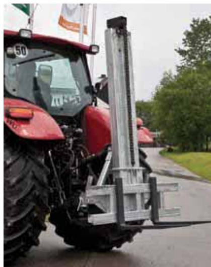
Hydraulic lifting frame with 900 mm forks
