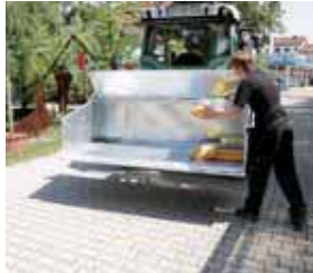
Especially sturdy design featuring rectangular pipe on the front of the rear bucket
