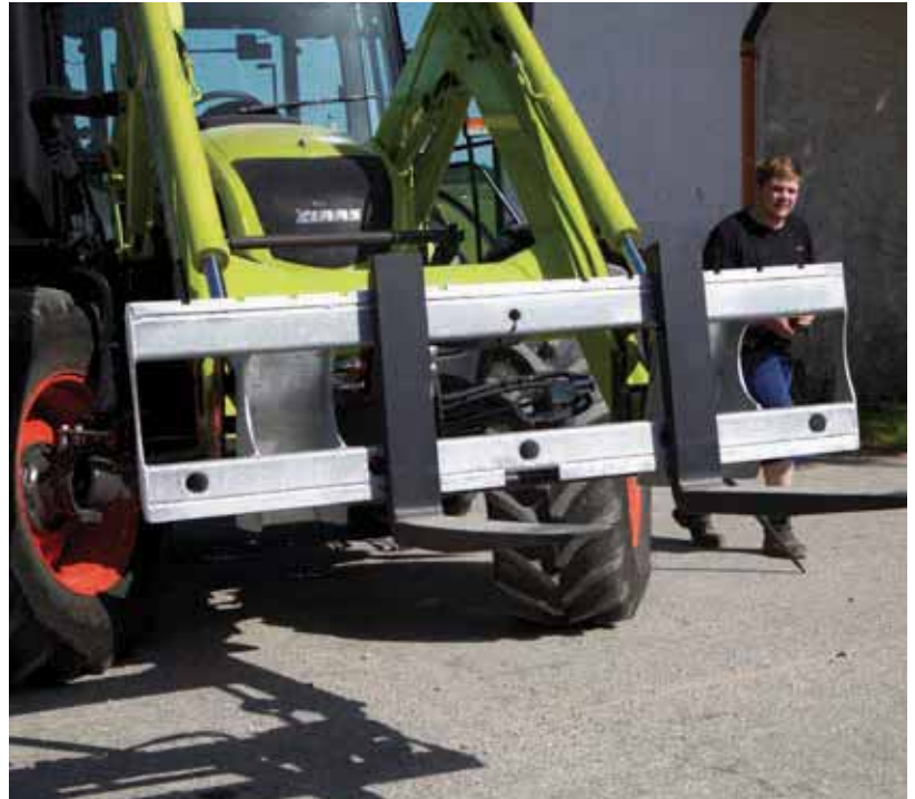
Very easy setup when using round bale tines due to available taper bushings (screw-on). With more or fewer tines depending on use.
