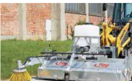
KEH type 500 on the wheel loader with spraying device, side brooms and heavy-duty support wheel
