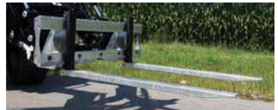
Adjustable mounting for round bale tines (heavy-duty tines; M28 x 1.5).
