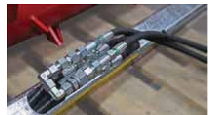
Hoses are routed internally, sturdy support pipes
