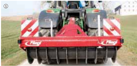
Illustration with warning sign set, optional for attachments with extra width
