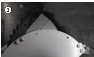
Screw conveyor fitted with blades
