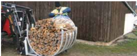
Professional batching directly on the device with wrap-round strap
