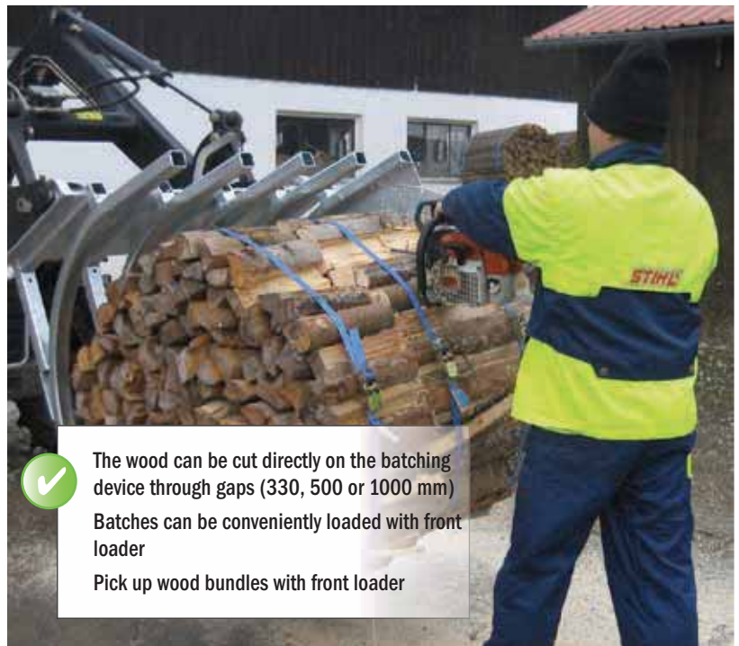
Professional batching directly on the device with wrap-round strap
