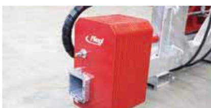
Counter weight (22 plates, 9.5 kg each)
