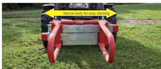
For square bales from 715 to 2450 mm, transport width: 1550 mm
