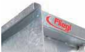
Especially sturdy design featuring rectangular pipe on the front of the rear bucket
