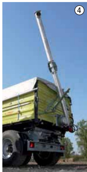
Can be inserted into Fliegl grain hatch 400 x 300 mm through swivel joint
