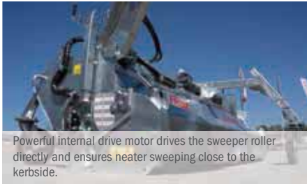
The sweeper machine comes standard with a hydraulic control block which is used to control free sweeping mode and the side brooms. Only 1 double acting connection is required. This ensures the hoses can be laid neatly.
