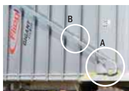
A) Raised by spring tension B) Individual length adjustment
