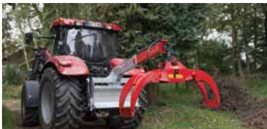
A specially developed pivot joint adjusts the gripper back to its starting point
