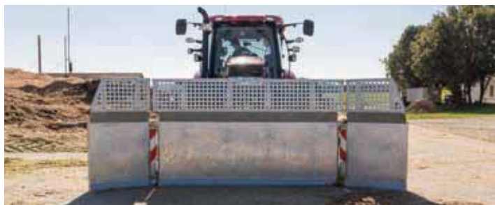
Wing can be swivelled back about 90°
