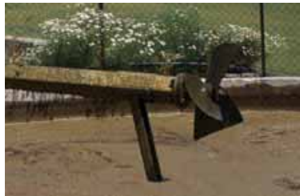
Agitator blade (Ø 500 mm standard, Ø 600 available for surcharge)
