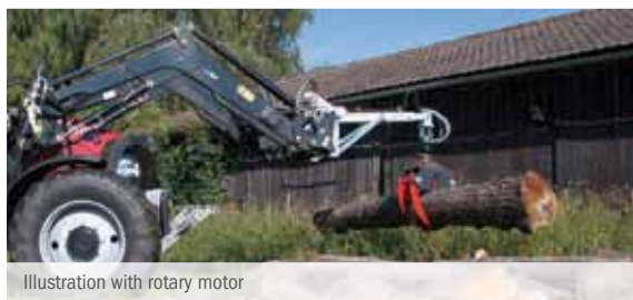
We offer matching electromagnetic switching valves for a 3rd and 4th oil circuit. No additional control valve is required for the gripper or rotary motor with this solution.
