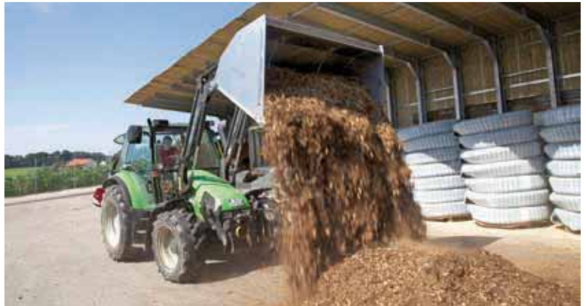
Fastened onto front loader with Euronorm quick exchange system
