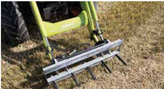
Very easy setup when using round bale tines due to available taper bushings (screw-on). With more or fewer tines depending on use.
