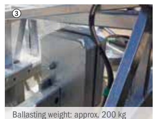
Ballasting weight: approx. 200 kg
