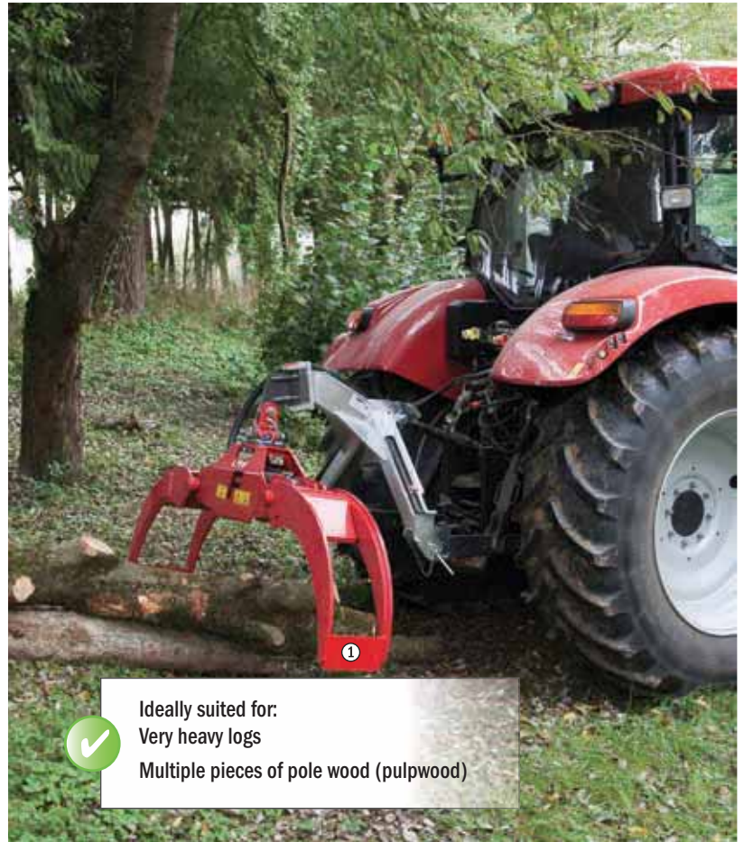
Loose, with hydraulic connections, without Euronorm mounting and three-point hitch
