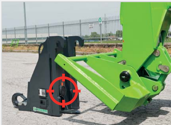
Sensor on the attachment.
