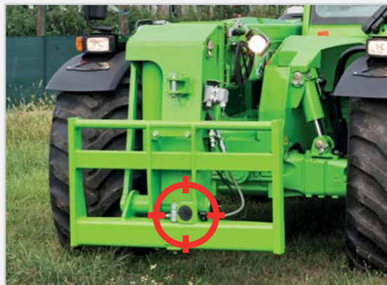
Sensor on the carriage.
